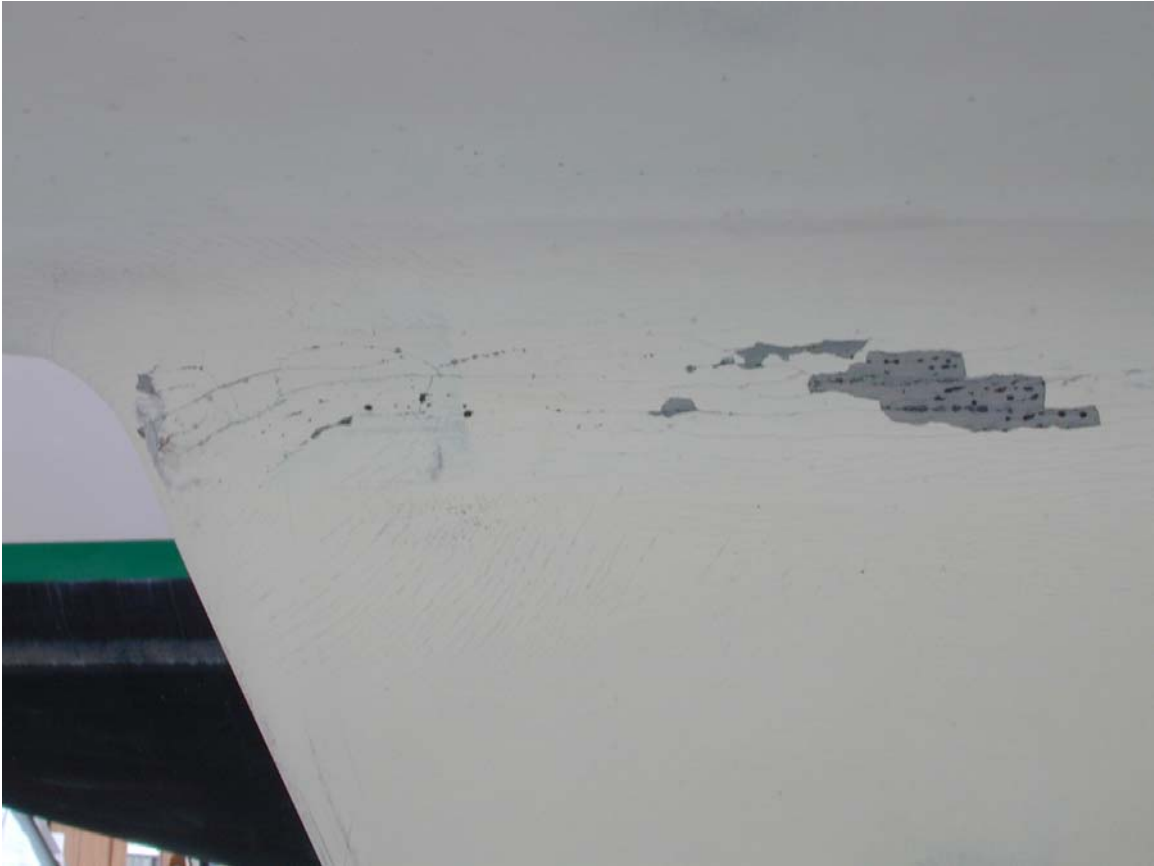
Severe fatigue cracking in a keel stub. This keel was close to falling off.
